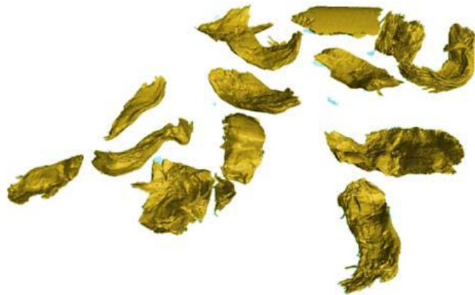
Figure 12 3D representation of wood particles by X-ray computed tomography.
