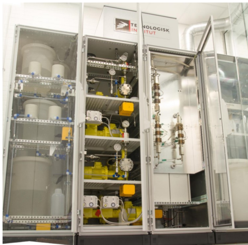
Figure 1. Photo of the supercritical flow reactor setup developed at DTI.
