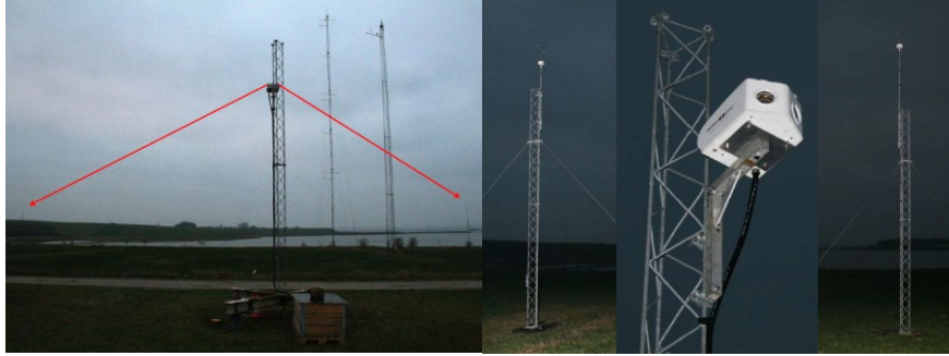
Fig. 5. Geometrical configuration of the field test at DTU Wind Energy in Roskilde to compare the performance of a WindEye prototype against reference sonic anemometers. The WindEye is facing a westerly direction. The field test covered three months of continuous operation (except for a few short-period fall-outs like power and software interruptions) during which the prototype was measuring the wind in various weather conditions (e.g. varying air humidity and temperature, and occasional rain). Figure 6 shows some results of the performance evaluation for LOS1 (data for 12 Jan 2014 13:00-14:00). Figure 7 shows the data for LOS2. Finally, Fig. 8 shows that the horizontal wind direction measured by the WindEye is in good agreement with those measured by the two reference sonic sensors (milestone M4). A more detailed discussion of these empirical results was presented in a recent lidar conference – M Sjöholm, E Dellwik, Q Hu, J Mann, C Pedersen, and PJ Rodrigo, 17 th International Symposium for the Advancement of Boundary-Layer Remote Sensing (Auckland, New Zealand, Jan 2014). A manuscript related to the detailed study of the field test data is to be submitted to a special issue of a remote sensing journal (milestone M5).
