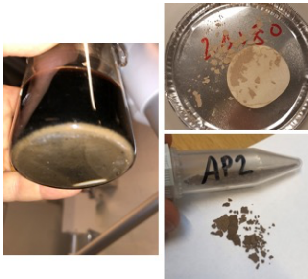
Figure 23: Mixing acidic wash water with precipitation chemicals (left). Diammonium phosphate (top right) and struvite (bottom right) product after filtering and drying.
