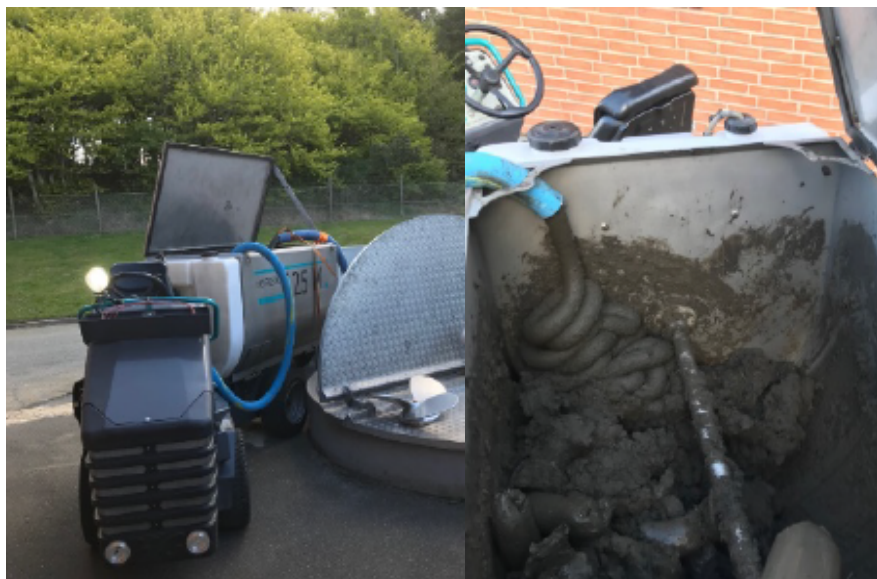
Figure 12: Left: Collection of sludge at the waste water treatment plant using the sludge wagon, Right: Conveying sludge at the pilot plant at Aalborg University.
