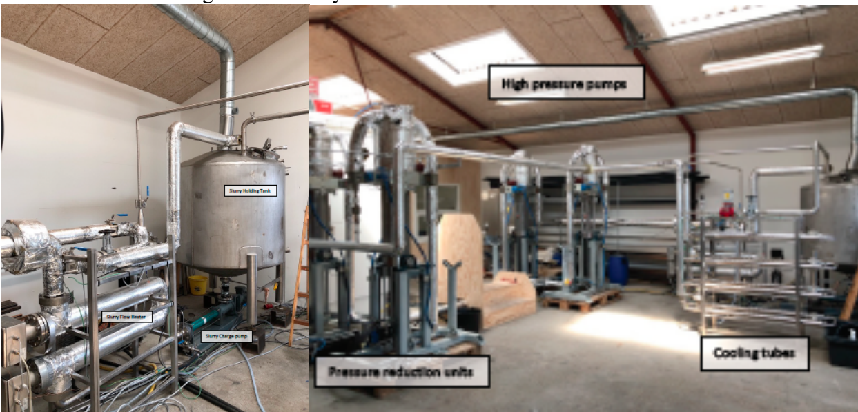
Figure 5: Photos of experimental set-up for wear testing of high pressure pump & pressure reduction pump.
