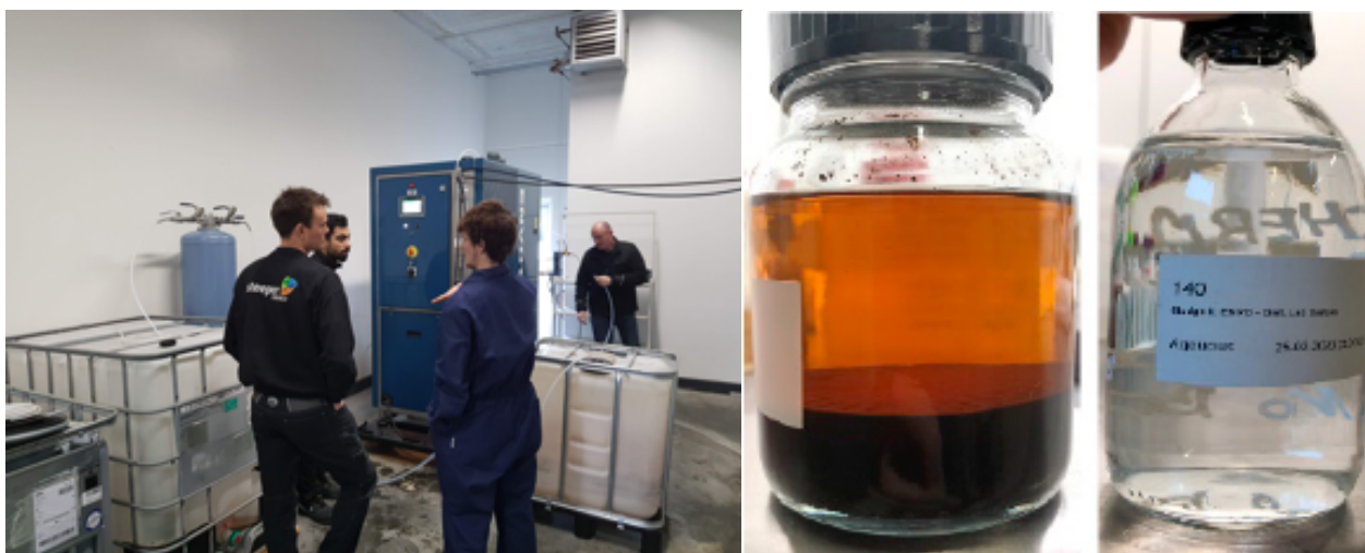
Figure 16: Left: Pilot test of recovery unit at Envotherm, Middle: Product sample with a water phase on the top and a bottom oil sand emulsion on the bottom, Right: Water effluent (distillate phase) after recovery unit.
