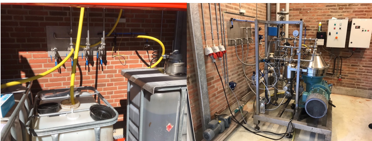
Figure 15: New disc bowl centrifuge set-up for product at Aalborg University.
