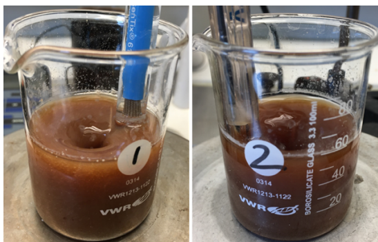
Figure 24 Aqueous phase samples during the treatment process for the phosphate recovery with (1) CaCl 2 and (2) CaO.
