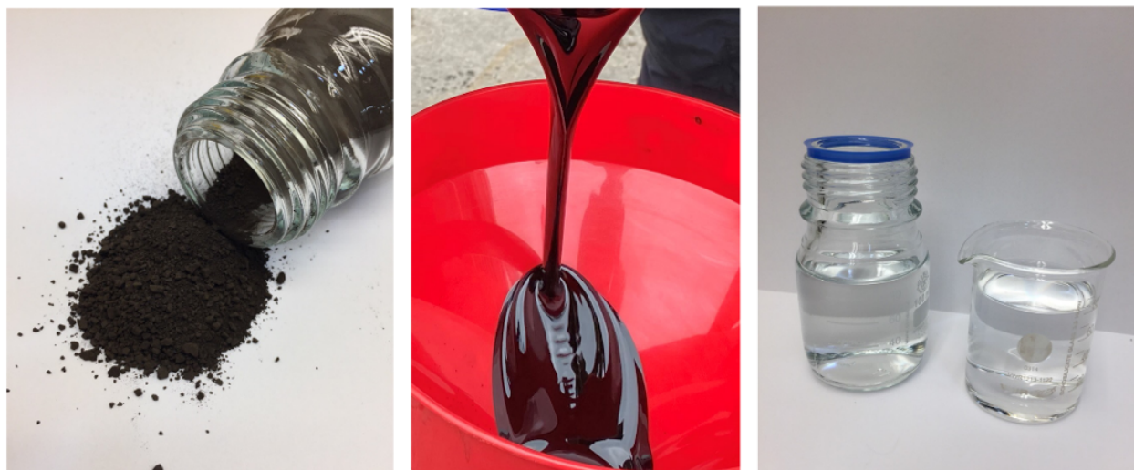
Figure 18: Photos of products from Hydrofaction ® of sewage sludge. Left: Solid product. Middle: sewage oil. Right: Water effluent.
