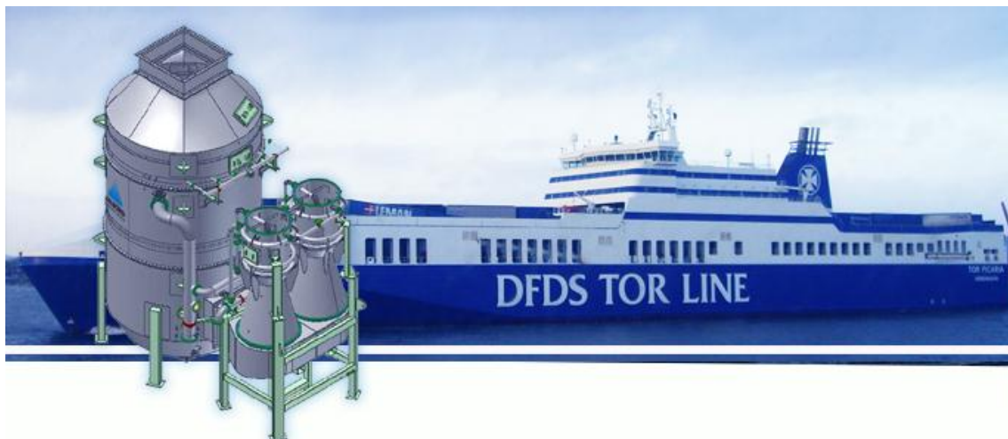
Figure 30. Ficaria Seaways Equipped with Presumably World’s Largest Retrofit Scrubber in 2009 (Picture: Alfa Laval)
