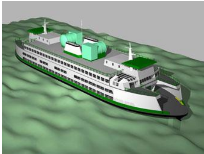
Figure 23. LNG tanks on top deck of WSF Issaquah Class ferry
