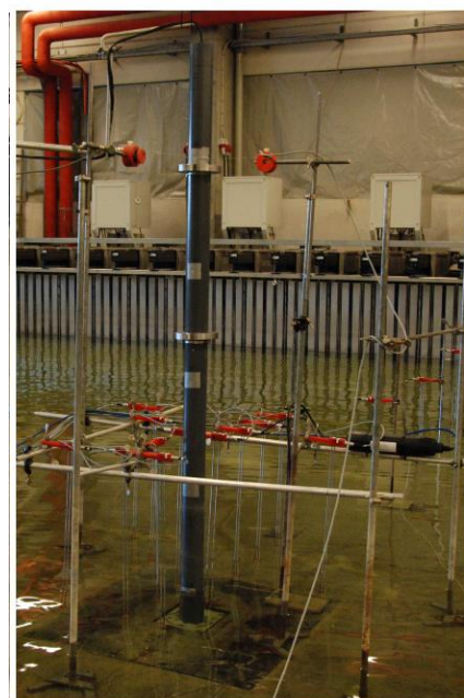
Figure 1: Test setup from the WaveLoads project at DHI. Left: Side view. Numbers show distances in lab scale in unit of meters. Right: Photo of the setup with the flexible monopile, point masses and the wave maker behind.
